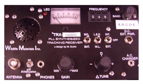
ANTENNA JACK: Accepts any 50 ohm coaxial cable with a BNC plug. To insert plug, push in jack and give a slight twist to the right.
