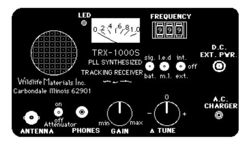
ANTENNA JACK: Accepts any 50-ohm coaxial cable with a BNC plug. To insert plug, push in jack and give a slight twist to the right.
